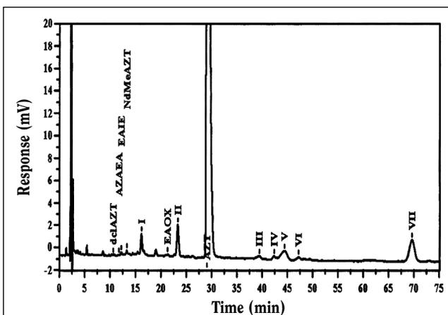
**Figure 2.** Typical chromatogram of an AZT bulk sample (concentration = 4.0 mg/mL) obtained under optimal chromatographic conditions. The column used was an XTerra RP18 5  $\mu$ m (25-cm  $\times$  4.6-mm i.d.) at 70°C. The mobile phase was ACN-pH 6.5 0.2M  $K_2HPO_4$ -water (35:10:55, v/v/v). The flow rate was 1.0 mL/min, the volume injected 100  $\mu$ L (total mass injected = 400  $\mu$ g), and the UV detection was set at 215 nm. Components I-VII are unknown.
